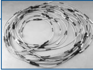
ARINC 629 Cable with Cable Couplers
