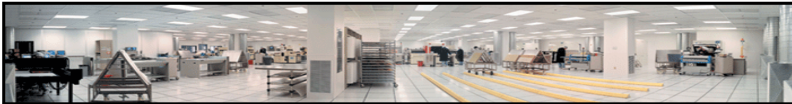
14,000 square foot, Class 10,000 clean room
