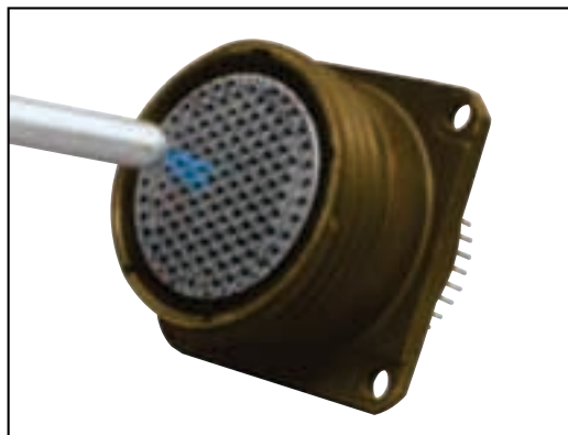
ESD Testing on MIL-DTL-38999, Series III Filter Cylindrical Connector (Actual Photo)
