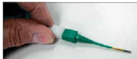
Plastic tool with contact in proper position.
