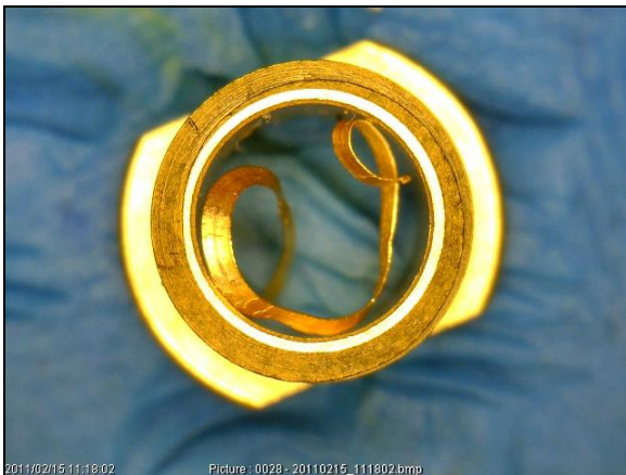
Figure 10: Rejectable Plated over chip from machining blocking functional inner diameter of the contact
