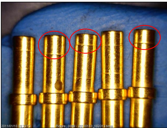
Figure 4: Rejectable Crimp well diameter violates print dimensions for the feature in the reduced diameter area.
