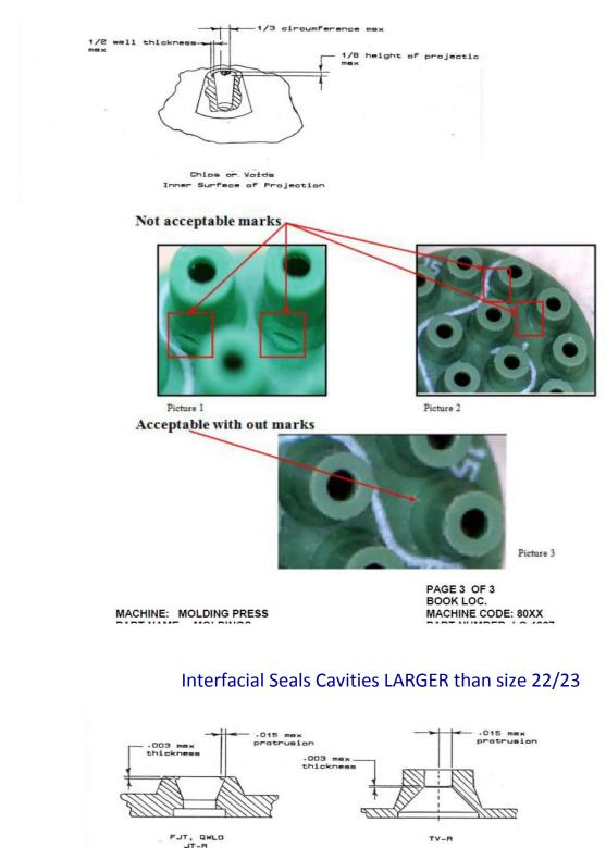
PR-302 Interfacial Seal, size 22/23 cavity holes 12/04/2013
