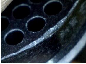
Not Acceptable. Cracks in insert
