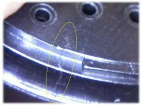
Not Acceptable. Cracks in insert
