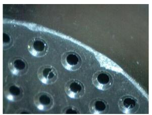
Not Acceptable. Cracks in insert
