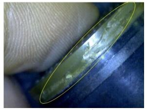
Not Acceptable. Torlon with Sinking after turn operation
