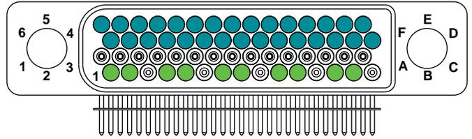
60 Pin Body with 5 Differential Pair, 30 Signal Contacts
