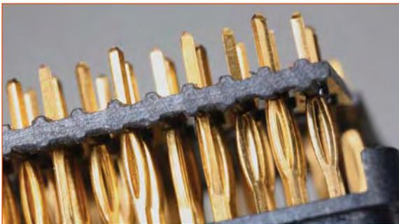
LRM backplane insert with compliant pins
