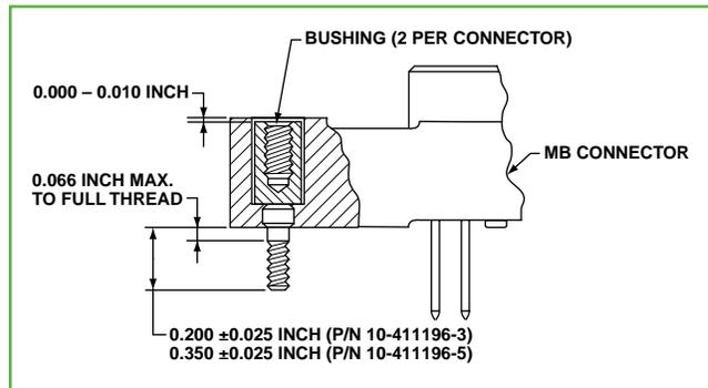
FIGURE 1: ASSEMBLY OF LOCKING/MOUNTING BUSHING INTO MB CONNECTOR
