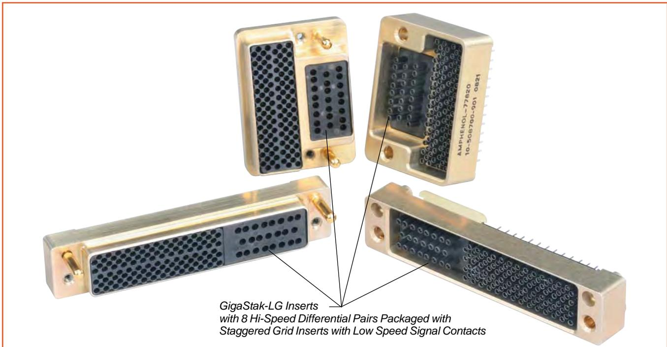
GigaStak-LG Inserts with 8 Hi-Speed Differential Pairs Packaged with Staggered Grid Inserts with Low Speed Signal Contacts
