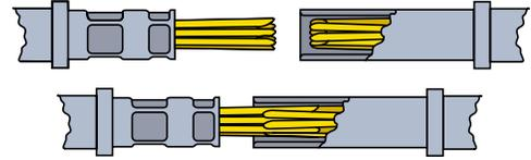
Multiple strands of high tensile strength wire bundled together to form brush-like contacts. See Brush Contact Technology section of this catalog for further description.
