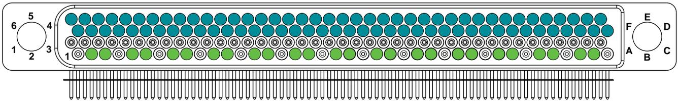
160 Pin Body with 13 Differential Pair, 80 Signal Contacts
