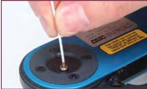
2. Insert contact into tool (use proper crimping tool as listed on preceding page). Crimp contact to wire. Tool will not open if contact is not fully crimped.
