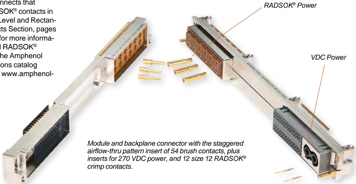
Module and backplane connector with the staggered airflow-thru pattern insert of 54 brush contacts, plus inserts for 270 VDC power, and 12 size 12 RADSOK® crimp contacts.
