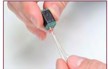
Snap the extraction end (white end) of the tool over the wire of the contact selected for removal. Carefully push the tool into the full depth of the contact cavity releasing the contact retaining collet. Hold the wire against the serrations on the tool, and withdraw the tool and the wired contact from the module.
