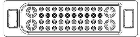
**Hybrid: 30 B<sup>3</sup> brush contacts, 10 size 12 power/coax/twinax contacts**
