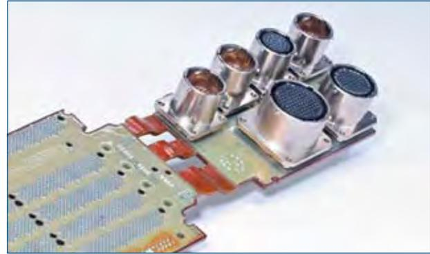
Cylindrical Connectors on PC Board
