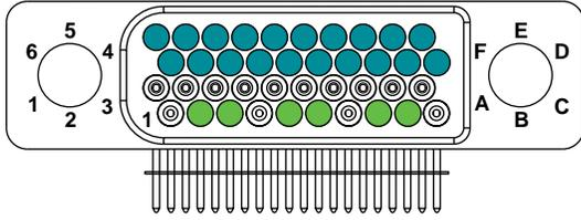
40 Pin Body with 3 Differential Pair, 20 Signal Contacts
