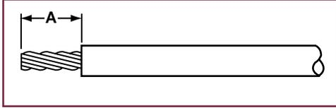
Strip wires to dimension "A" shown in table at right. Avoid cutting or nicking wire strands.
