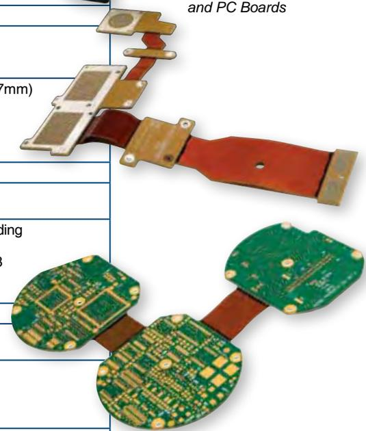
Flex circuitry is used in a wide variety of Amphenol board level and rectangular interconnects, as shown throughout this catalog:
