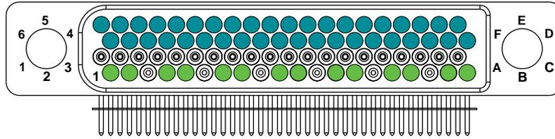
80 Pin Body with 7 Differential Pair, 40 Signal Contacts
