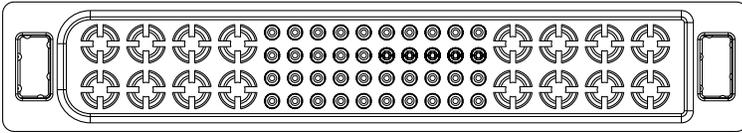
**Hybrid: 40 B<sup>3</sup> Brush contacts, 4 size 16 power/coax/twinax contacts**
