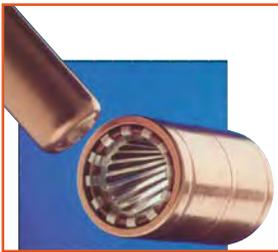
The RADSOK® socket cylinder within female contact has several equally spaced longitudinal beams twisted into a hyperbolic shape. As the male pin is inserted, axial members in the female half deflect, imparting high current flow across the connection with minimal voltage loss. The hyperbolic, stamped grid configuration ensures a large, coaxial, face-to-face surface area engagement.
