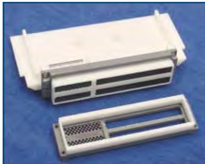
Heat Sink and LRM Connector Prototype
