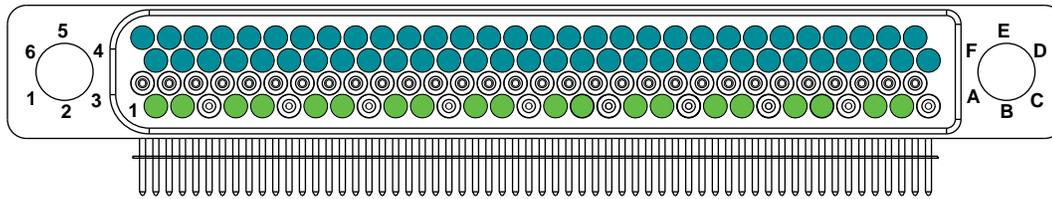
120 Pin Body with 10 Differential Pair, 60 Signal Contacts
