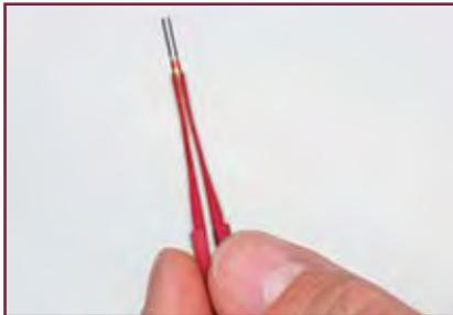
Using proper insertion/removal tool as listed on previous page, slip wire into insertion end (colored end), placing crimp end of contact inside the slotted portion and contact shoulder against end of tool.
