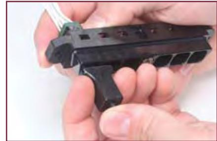
With the module removal tool fully inserted, push the extraction plunger to eject the module out of the rear of the connector.
