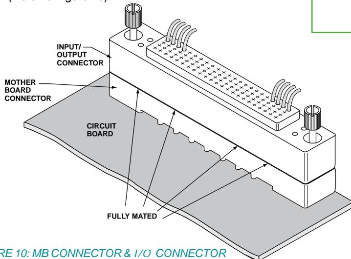
FIGURE 10: MB CONNECTOR & I/O CONNECTOR FULLY MATED CONDITION
