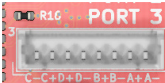
Figure 2: Mapping of ethernet signals onto PicoBlade connectors.
