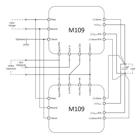
Note: Parallel operation via output voltage droop. Voltage regulation is ±2%.
