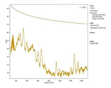
CE102 MIL-STD-461F Conducted Emission, 10 kHz -150 kHz
