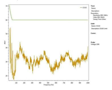
CE102 MIL-STD-461F Conducted Emission, 150 kHz -10 MHz Return (nominal input voltage, full load)
