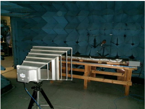
RE102 Test, 200MHz-1GHz, Vertical, Position 2
