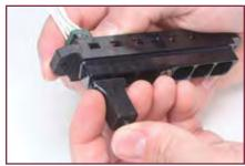
With the module removal tool fully inserted, push the extraction plunger to eject the module out of the rear of the connector.
