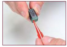
Align contact with the cavity at the rear face of the module. Carefully push the contact into the full depth of the cavity. Withdraw tool. A slight axial pull on the wire will confirm contact is locked in proper position.
