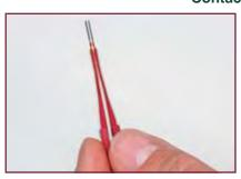
Using proper insertion/removal tool as listed on previous page, slip wire into insertion end (colored end), placing crimp end of contact inside the slotted portion and contact shoulder against end of tool.
