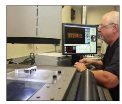
Checking for dimensional accuracy of LRM parts and heatsinks.
