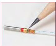
1. Fully insert wire into contact crimp pocket. Wire must be visible through wire inspection hole.
