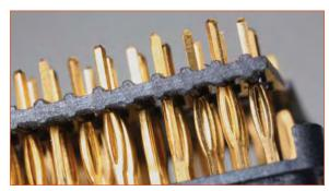
LRM backplane insert with compliant pins
