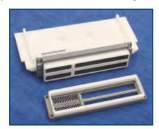
Heat Sink and LRM Connector Prototype
