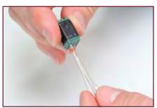
Snap the extraction end (white end) of the tool over the wire of the contact selected for removal. Carefully push the tool into the full depth of the contact cavity releasing the contact retaining collet. Hold the wire against the serrations on the tool, and withdraw the tool and the wired contact from the module.
