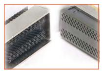
Staggered Grid Airflow-thru pattern - in a module on right, and in a backplane on left. Note the increased spacing in the center. This is designed for wider board packages, and accommodates airflow-thru heatsinks. (See illustration on page 18).
