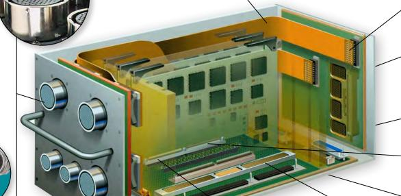
Designed to meet the high-density needs of today's integrated electronic modules, this straddle-mount connector uses the Bristle Brush contact, a proven military avionics solutions that meets MIL-DTL-55302 requirements. The low mating force, extended service life and stable electrical performance of the Brush contact enables the performance demanded by Line Replaceable Module (LRM) applications. Hybrids available with fiber optics and high power RADSOK®.
