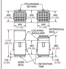
**Sealed Socket** Sealed Pin Module Module Part number: Part number: LMD-4003-S LMD-4003-P
