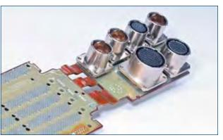
Cylindrical Connectors on PC Board
