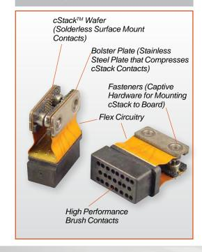
Low Mating Force MIL-DTL-55302 Coax/Fiber Optics Accessories/Install
