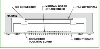
FIGURE 4: TYPICAL FIXTURE FOR SOLDERING MB CONNECTORS
