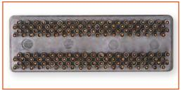
Staggered grid airflow-thru backplane insert.
