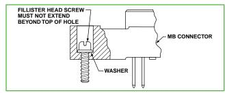
FIGURE 3: MB CONNECTOR WITH SCREW MOUNTING
