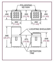
**Socket** Pin Module Module Part number: Part number: LMD-3001-P LMD-3001-S
