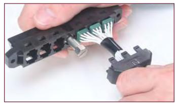
Tape wire bundle in area of cable clamp, and build up diameter to approx. 3/8 inches, if required. Align self-locking tines of the strain relief housing with the cavities adjacent to each module. Push the strain relief housing into place until the self-locking tines snap and lock strain relief into position. Assemble opposite half of strain relief housing to connector and tighten tie-strap to provide clamping force on the wire bundle.
