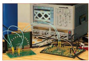
Test bench for LRM connectors. Computer screen shows a pass/fail mask test eye diagram.
