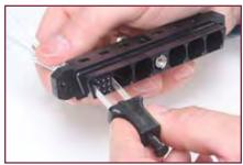
Select module to be removed and place the blades of removal tool into the removal slots at the front of the connector. Push the removal tool into the full depth of the cavity, releasing the module retention tines.
