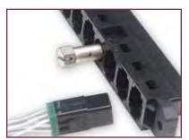
Align the module with the proper cavity at the rear of the housing. The module keyway must be positioned to accept key in housing cavity. Carefully insert the module straight in to the cavity until fully seated and locked in place. A slight axial push on the front of the module or a pull on the cable bundle will confirm module is locked in proper position.
