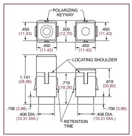
Socket Pin Module Module Part number: Part number: LMD-3004-S LMD-3004-P
