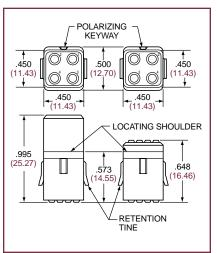
**Socket** Pin Module Module Part number: Part number: LMD-3005-S LMD-3005-P
