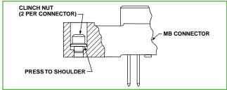
FIGURE 2: MB CONNECTOR WITH CLINCH NUT MOUNTING
