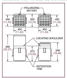
Socket Pin Module Module Part number: Part number: LMD-3003-S LMD-3003-P
