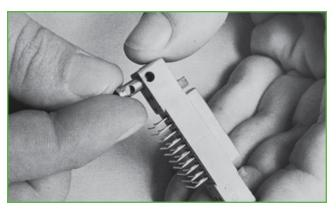
LOCKING BUSHING ACCESSORY INSERTED INTO PC CONNECTOR BODY
