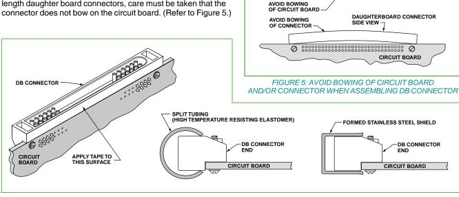
FIGURE 6: THREE TYPICAL MASKING APPLICATIONS FOR SOLDERING DB CONNECTORS
