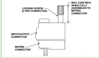
FIGURE 9: I/O LOCKING SCREW DIMENSIONS
