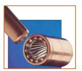
The RADSOK® socket cylinder within female contact has several equally spaced longitudinal beams twisted into a hyperbolic shape. As the male pin is inserted, axial members in the female half deflect, imparting high current flow across the connection with minimal voltage loss. The hyperbolic, stamped grid configuration ensures a large, coaxial, face-to-face surface area engagement.
