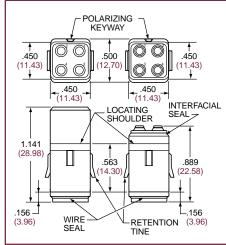
**Sealed Socket Sealed Pin** Module Module Part number: Part number: LMD-4005-S LMD-4005-P
