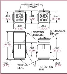
**Sealed Socket** Sealed Pin Module Module Part number: Part number: LMD-4001-P LMD-4001-S
