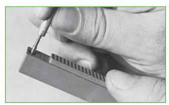
LOCKING SCREW ACCESSORY INSERTED INTO IO CONNECTOR BODY
