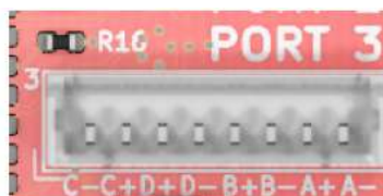
Figure 7: Mapping of ethernet signals onto PicoBlade connectors.
