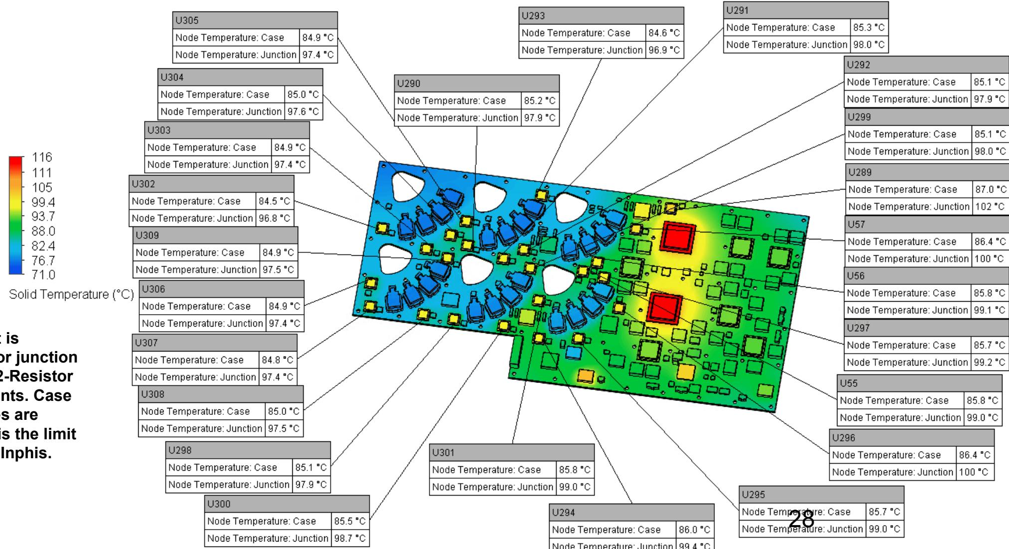
Note: Surface plot is showing internal or junction temperatures for 2-Resistor network components. Case temperature values are shown since this is the limit type specified for Inphis.
