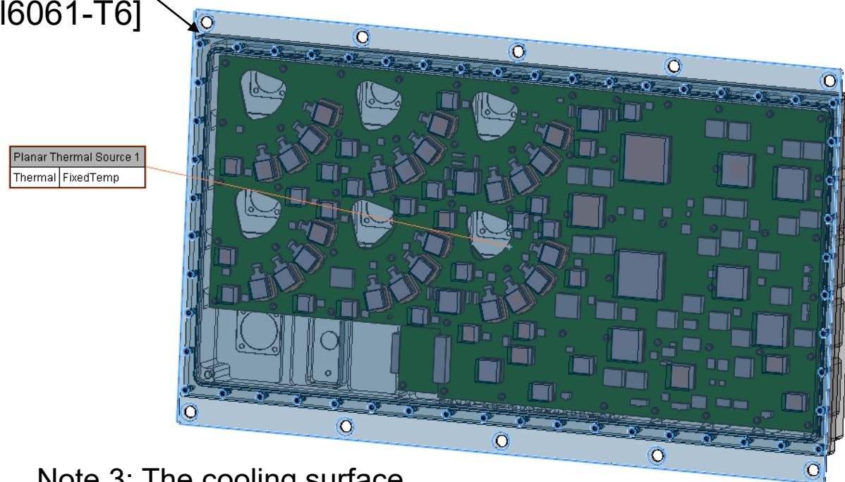
Note 3: The cooling surface (= rear cover outer surface) temperature is fixed in the thermal simulation. The value is chosen as the operating ambient temperature.
