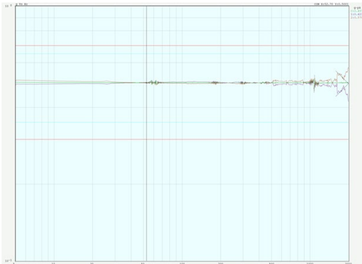
X axis Sine Sweep Whole assembly
