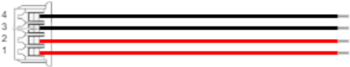
Voltage input cable pinout (red= 5V, black = GND)
