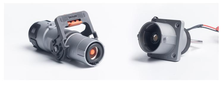
Voltarius is a high power interconnect optimized for higher voltages. This connector series was designed to provide performance up to 1000Vdc and 450A with proven RADSOK® technology. It also provides essential safety features such as interlock circuitry and a secondary locking mechanism.
