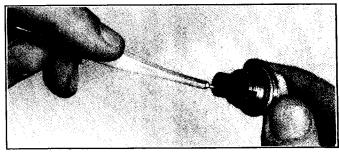
Press the wire of the contact to be removed against the serrations of the plastic tool and pull both the tool and the contact wire assembly out of the connector.
